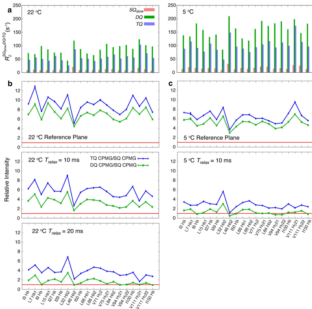
Fig. 6 Relative sensitivities of methyl ^1\text{H} SQ, DQ and TQ CPMG datasets recorded on a wild-type T4L sample ( \sim 18 kDa) that does not undergo chemical exchange. a Relaxation rates for DQ coherences are significantly larger than for the TQ and the \text{SQ}_{\text{slow}} coherences. b Relative intensities of peaks in the reference plane ( T_{\text{relax}} = 0 ) and in planes with \nu_{\text{CPMG}} = 2000 Hz and T_{\text{relax}} = 10 or 20 ms for the SQ, DQ and TQ CPMG experiments recorded at 22 °C ( \tau_c \sim 11.7 ns).
