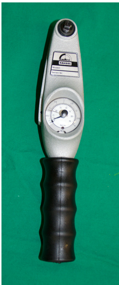
Fig. 2 Torque meter, Gedore Torque Tech. The shown torque meter has a measuring range of 0–4 Nm. A second device was used in the study with a range of 0–20 nm
