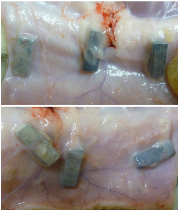
Fig. 5 The top panels shows the implant sites of the magnesium implants after successful anchoring in the subcutaneous fascia whilst the lower panel illustrates migration that occurred in the subcutaneous layer during the period of implantation
