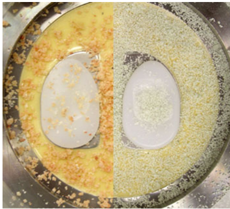
Fig. 1 Third-body debris in the test chamber without test fluid. On the left side the bone fragments and on the right side the cement debris is shown
