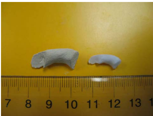
Fig. 8 As-fabricated green and sintered 3DP-HAAW model of mandibular bone
