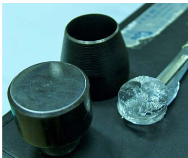
Fig. 1 A typical hydrogel samples tested in compression
