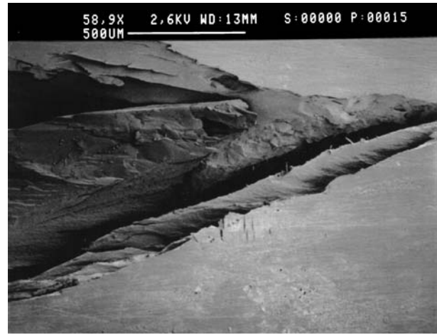
Figure 9 Composite processed for two minutes at 125 °C. The tensile surface is shown.
