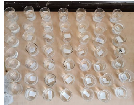
Fig. 5 Immersion of samples in chemical solutions
