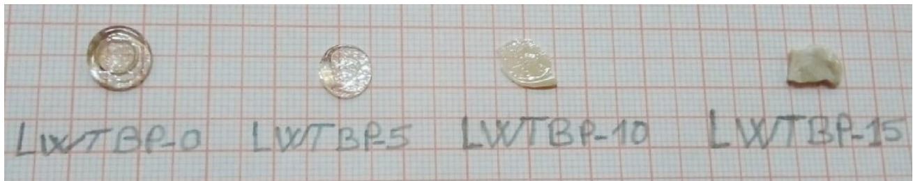
Fig. 1 Photo for transparent glasses (LWTBP-0 and LWTBP-5) and opaque glasses (LWTBP-10 and LWTBP-15)
