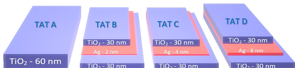
Fig. 1 3D diagram depicting TiO 2 /Ag/TiO 2 multilayer film with different Ag thickness
