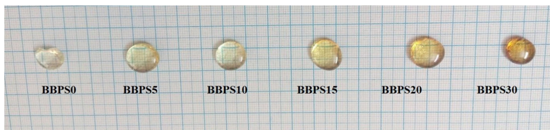
Fig. 1 An image of the prepared BBPS0–BBPS30 glass samples
