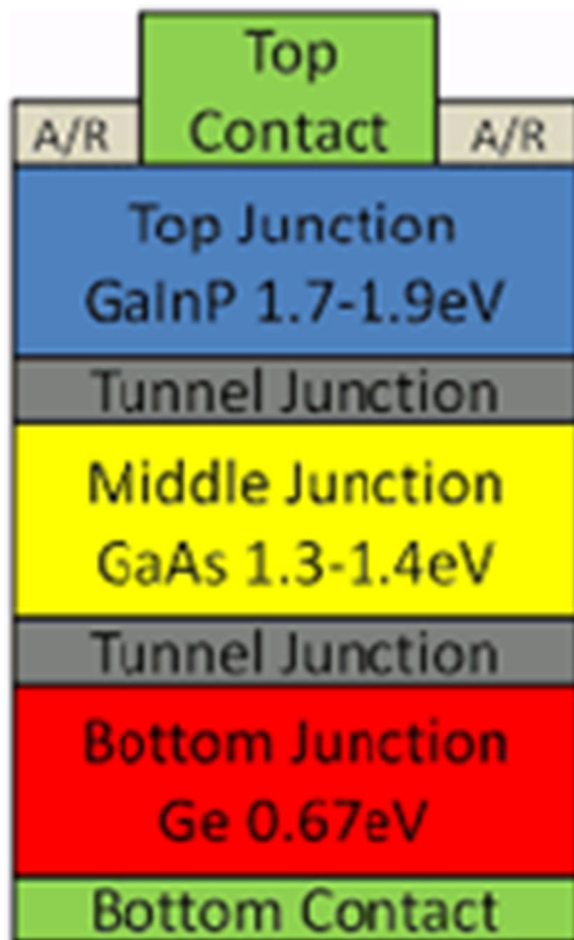
Fig. 1 Typical multijunction solar cell structure
