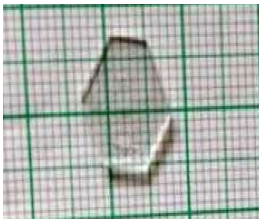
Fig. 1 The photograph of the grown CPMTC crystal
