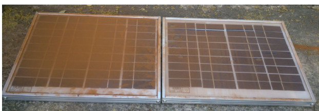
Fig. 20 Property comparison of coated and uncoated module (with dust deposition)
