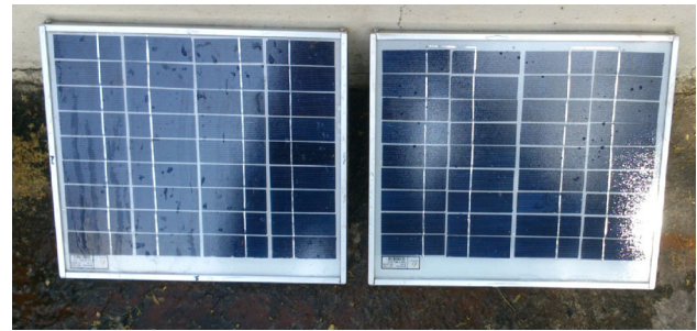
Fig. 21 Property comparison of coated and uncoated module on PV module (After cleaning the surface with water)
