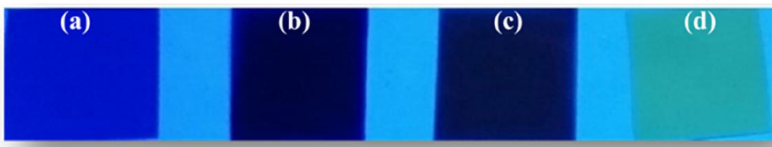
Fig. 9 Photographs of a PMMA, b PMMA/ZnO, c 0.1 wt% and d 0.25 wt% CBPEA dye-doped PMMA/ZnO polymer nanocomposite films under UV lamp of 365 nm
