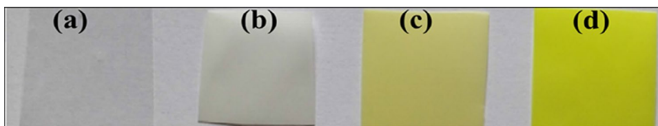
Fig. 1 Photographic images of a PMMA, b PMMA/ZnO, c 0.1 wt% CBPEA, d 0.25 wt% CBPEA nanocomposite films
