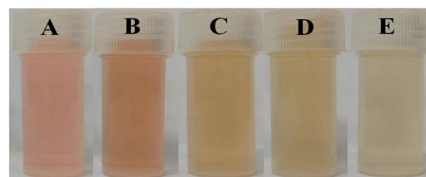
Fig. 9 Degradation time-resolved UV-Vis spectra and optical images of eosin yellow degradation by gold NPs in the presence of \text{NaBH}_4 . Reaction conditions: [Eosin yellow] = 2.0 \times 10^{-5} mol dm -3 , [gold NPs] = (3.4 \times 10^{-4}) mol/L, [ \text{NaBH}_4 ] = 3.4 \times 10^{-3} mol dm 3 (Color figure online)
