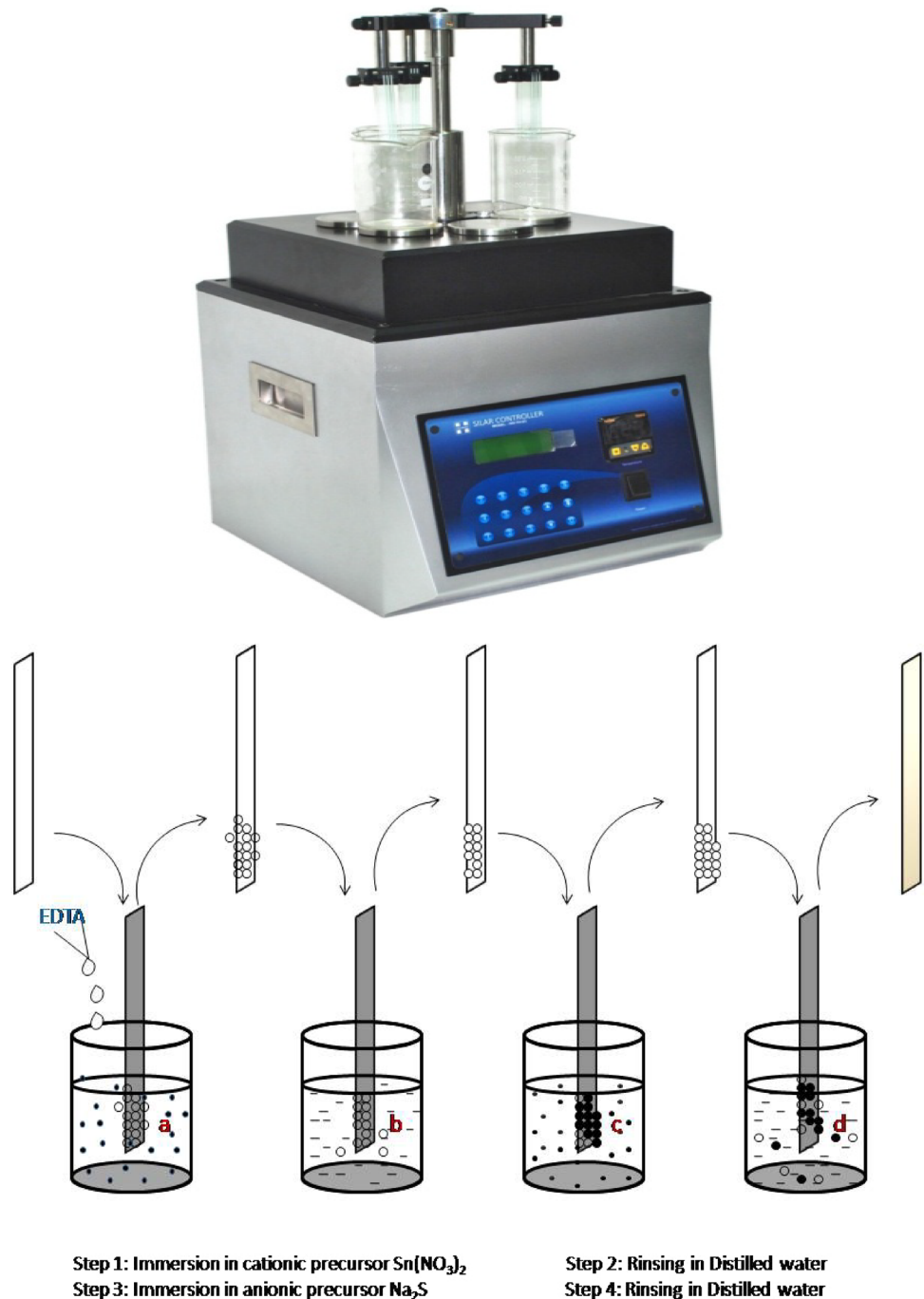
Fig. 1 Schematic representations of SILAR deposition for SnS thin films with EDTA
