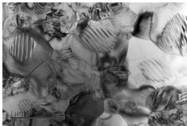
Fig. 4 TEM micrographs of 9010BTBNT ceramic samples doped with 1.5 mol% \text{Ta}_2\text{O}_5 (Color online)
