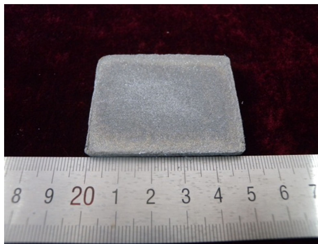
Fig. 4 The fabricated composite in the application of heat dissipation prepared by LSS process
