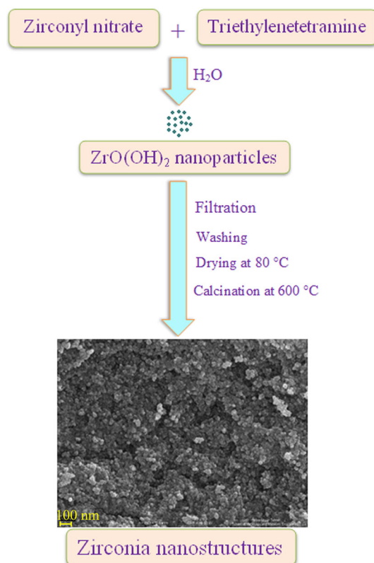
Fig. 1 Schematic depicting the preparation of nano zirconium dioxide powders
