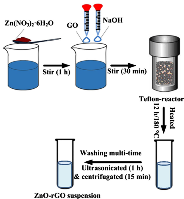
Fig. 1 Preparation of ZnO–rGO suspension via hydrothermal treatment
