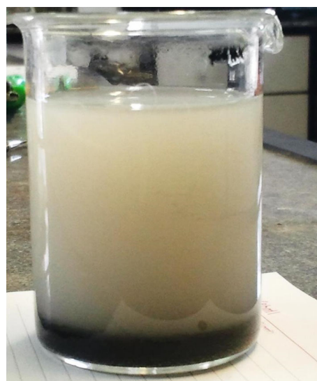
Fig. 3 Separation of suspension during the EPD process of CNTs and ZnS:Mn nanoparticles
