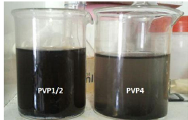
Fig. 6 Macro image of CNT–ZnS:Mn suspensions with different PVP:CNT weight ratios a 0.25 and b 4
