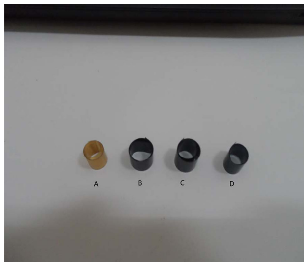
Fig. 7 Digital images of pure PEN and the \text{Al}_2\text{O}_3/\text{MWCNTs}/\text{PEN} micro-nanocomposite films which were curled into cylinders: A, B, C and D correspond to pure PEN film, composite films with 1, 3 and 7 wt% MWCNTs particles, respectively
