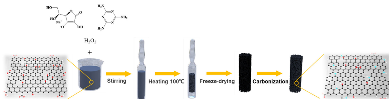
Figure 1 Scheme of the synthetic procedure for the preparation of the rGO/melamine porous aerogel.
