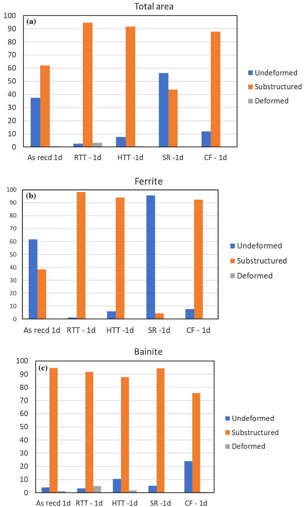
Figure 12 a Fraction of recrystallized, substructured or deformed grains in total area (1d in the labels denotes that the subgrain boundary threshold was 1°), b fraction of recrystallized, substructured or deformed grains in ferrite (1d in the labels denotes that the subgrain boundary threshold was 1°) and c fraction of recrystallized, substructured or deformed grains in bainite (1d in the labels denotes that the subgrain boundary threshold was 1°).
