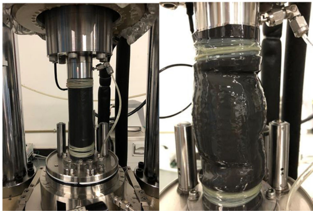
Figure 18 Triaxial test specimen.
