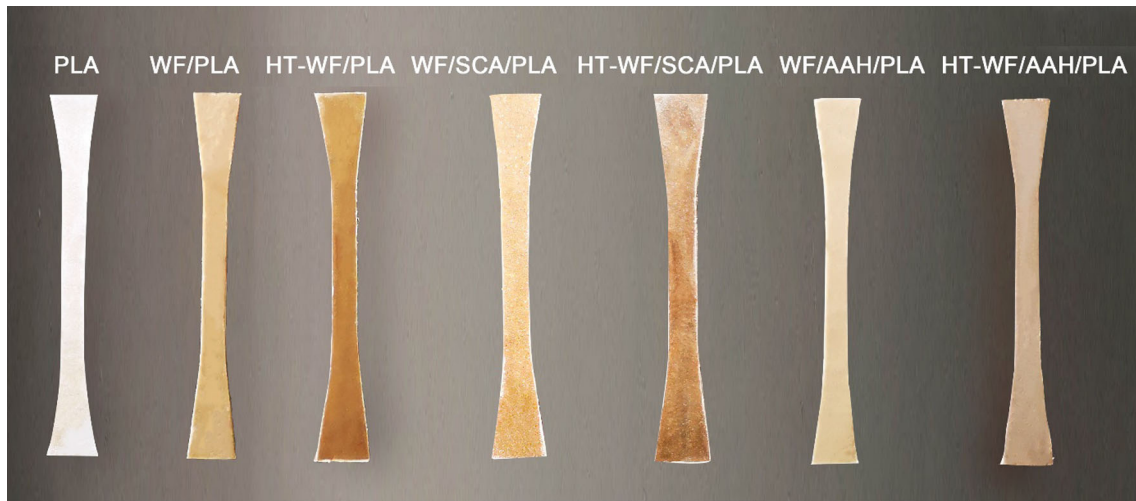
Figure 6 Appearance of the composites with different modifications.
