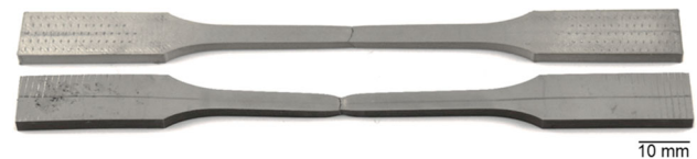
Figure 12 Photographic image of both fractured SS316L sintered tensile specimen (top) and SS316L wrought specimen (bottom) showing two types of necked regions.
