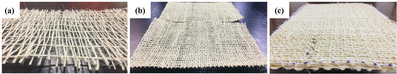
Figure 23 Various textile structure developed a UD Tows b 2D preform c 3D woven orthogonal structures.
