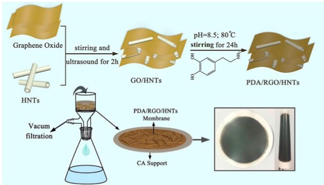
Figure 10 The preparation procedures of polydopamine (PDA)/RGO/HNTs membranes [120].
