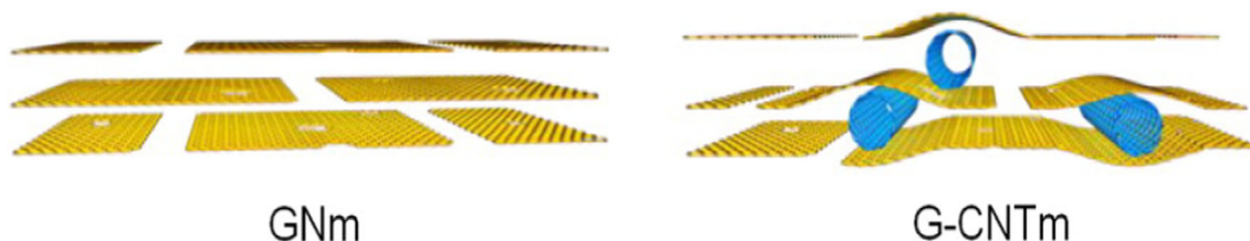
Figure 9 Schematic representation of the structure and water transport path for (left) graphene nanomembrane (GNm) and (right) graphene-carbon nanotube membrane (G-CNTm). [116].
