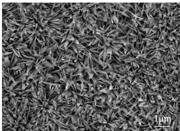
Figure 1 SEM images of boehmite films obtained by one-step hydrothermal reaction (reaction time 9 h, reaction temperature 190 °C).
