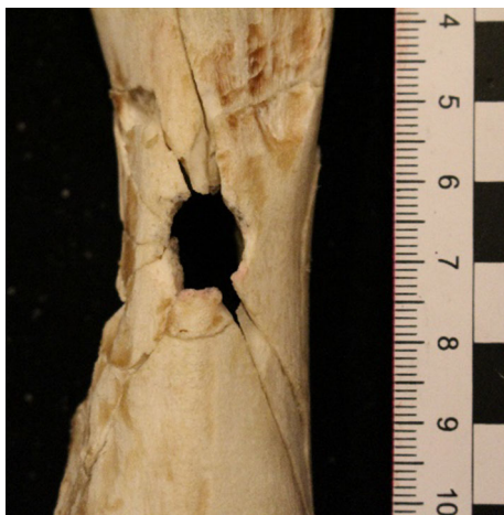
Figure 6 A porcine target impacted with a lead sphere.
