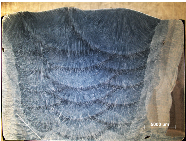
Figure 1 Macro-etched all-weld metal sample.
