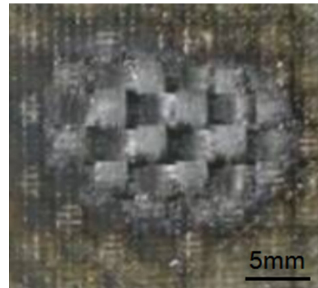
Figure 12 Macroscopic morphology of S1 rear surface after laser irradiation with energy of 1500 W for 10 s.
