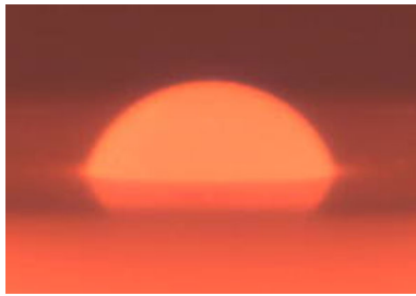
Fig. 2 Droplet of the liquid braze alloy A on alumina, 200 s after melting
