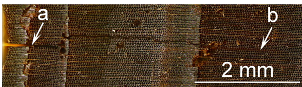
Fig. 2 Crack tip sharpened with a razor blade. Position of razor blade cut (a), crack propagated spontaneously to the point (b)
