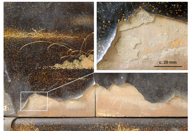
Fig. 4 Detail of typical coating loss on a nineteenth century Japanese export-type lacquer cabinet in the V&A collection (V&A 303-1876, courtesy of the Victoria and Albert Museum, London)
