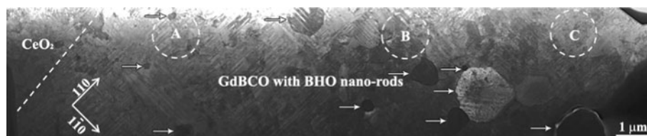
Fig. 7 Low magnification plan-view image of 2.9 \mu\text{m} -thick GdBCO layer containing BHO nano-rods. Left hand side corresponds to \text{CeO}_2 interface side and the opposite side to surface region
