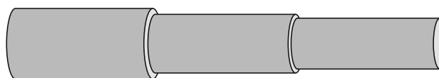
Fig. 1 Schematic drawing of a three-step profile bar after hydrogen charging and turning. After hydrogen charging, the bar is turned in sections. The left section is left intact while on the two sections to the right a thin layer is removed by turning. Each section is then divided into two pieces before the hydrogen content is determined
