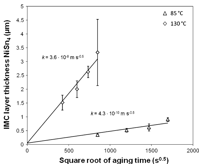
Fig. 5 IMC layer thickness of NiSn_4 versus square root of aging time for the temperatures 85 and 130 °C. The error bars represent the \pm standard deviation of four measurements of each specimen
