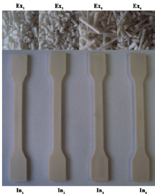
Fig. 3 Injected and extruded samples
