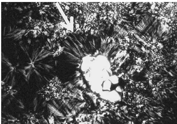
Fig. 10 Polarised optical microscopy picture of a microtomed cross section of the slowly cooled PP/flax composite sample, cut perpendicular to the fibre axis, showing the presence of a non-symmetrical transcrystalline layer developed around the fibre
