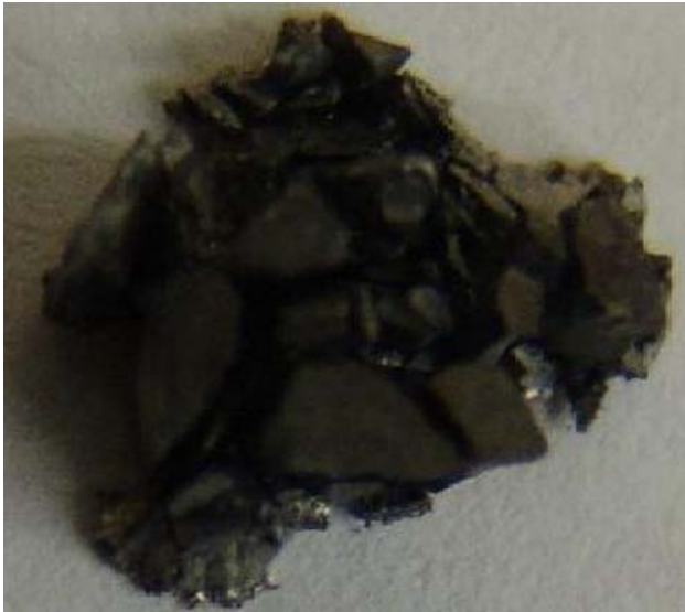
Fig. 12 Typical failed specimen during dynamic loading at elevated temperatures
