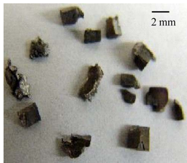
Fig. 8 A typical failed specimen at room temperature under dynamic loading
