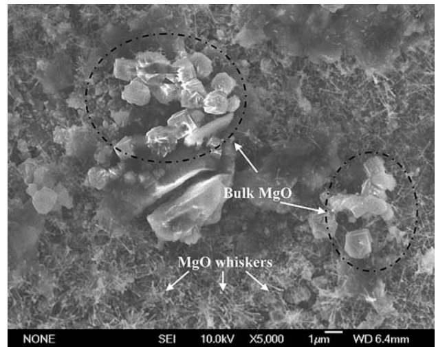
Fig. 5 SEM image of bulk MgO formed on the surface of bulk polycrystalline MgB 2 samples, where MgO vapor reached a medium supersaturation, at a temperature of 720 °C
