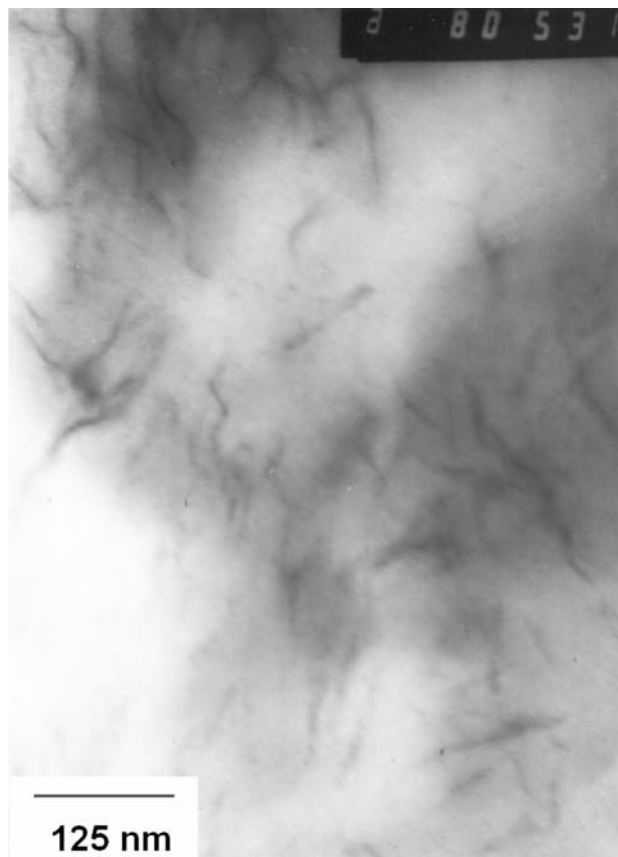
Fig. 2 TEM micrograph of the PE nanocomposite containing 1% by volume of MMT
