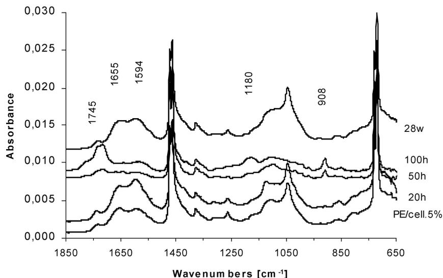
Figure 3 ATR Ge spectra of PE/Cell. (5%) film before photo-degradation, after 20, 50 and 100 h of UV-irradiation, and after 28 weeks of composting.
