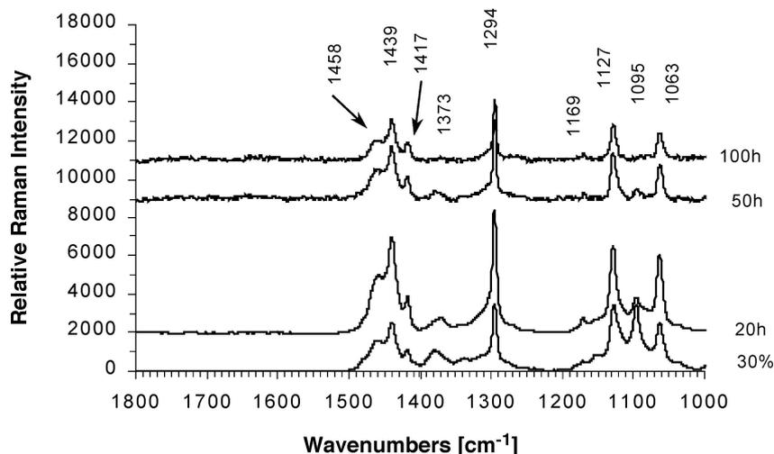
Figure 7 Raman spectra of PE blends with a 30% amount of cellulose before (30%) and after 20, 50 and 100 h UV-irradiation; the intensity of the 1294  $\text{cm}^{-1}$  signal has been used as normalization peak.
