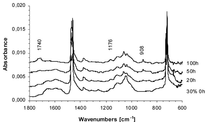
Figure 4 ATR Ge spectra of PE/Cell. (30%) film before photo-degradation, after 20, 50 and 100 h of UV-irradiation.
