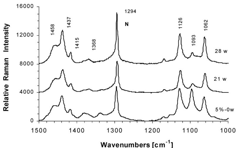
Figure 9 Raman spectra of PE blends with a 5% amount of cellulose before (0 w) and after 21 and 28 weeks of bio-degradation, respectively; the intensity of the 1294  $\text{cm}^{-1}$  signal has been used as normalization peak.
