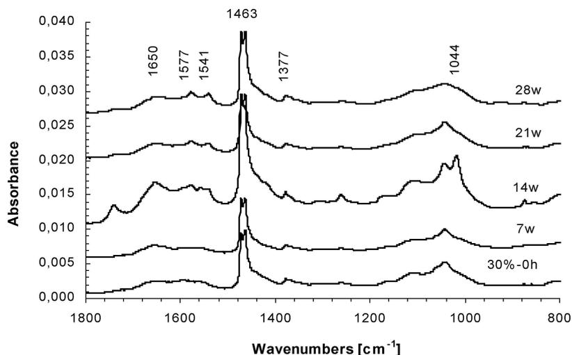
Figure 8 ATR Ge spectra in the spectral range 800–1800  $\text{cm}^{-1}$  of PE/Cell. (30%) film before bio-degradation (0 h) and after 7, 14, 21 and 28 weeks of composting, respectively.
