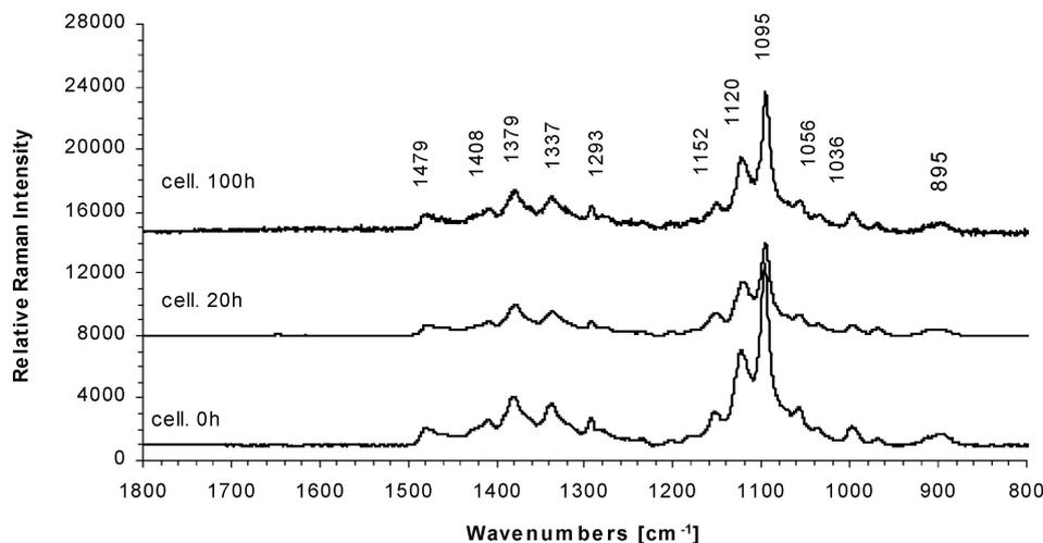
Figure 5 Raman spectra of cellulose powder before (0 h) and after 20 and 100 h of UV-irradiation; the intensity of the 1095  $\text{cm}^{-1}$  signal has been used as normalization peak.
