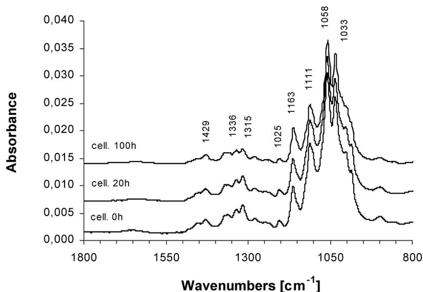
Figure 2 ATR Ge spectra in the range 800–1800  $\text{cm}^{-1}$  of cellulose powder before photo-degradation and after 20 and 100 h of UV-irradiation.
