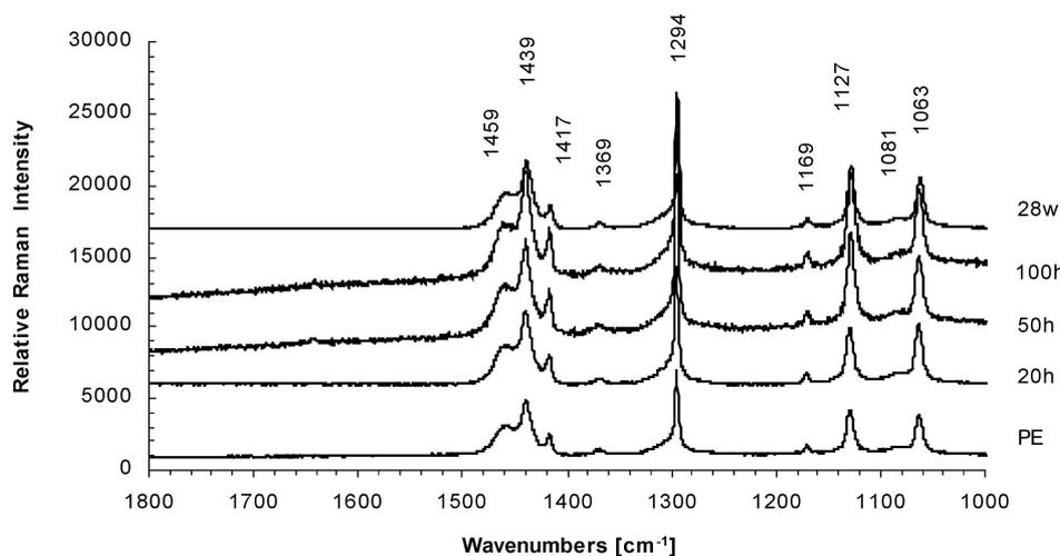
Figure 6 Raman spectra of polyethylene before (PE) and after 20, 50, 100 h of UV-irradiation and after 28 weeks of composting; the intensity of the 1294  $\text{cm}^{-1}$  signal has been used as normalization peak.
