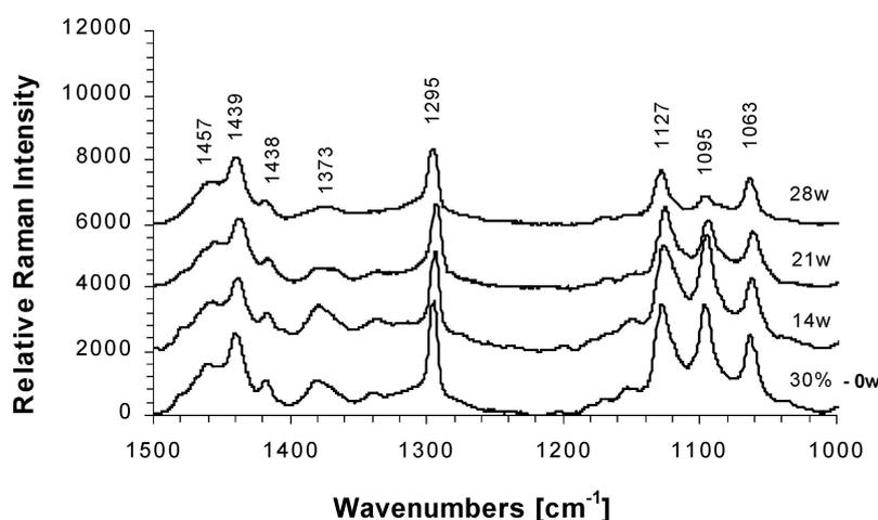
Figure 10 Raman spectra of PE blends with a 30% amount of cellulose before (0 w) and after 14, 21 and 28 weeks of composting, respectively; the intensity of the 1294  $\text{cm}^{-1}$  signal has been used as normalization peak.
