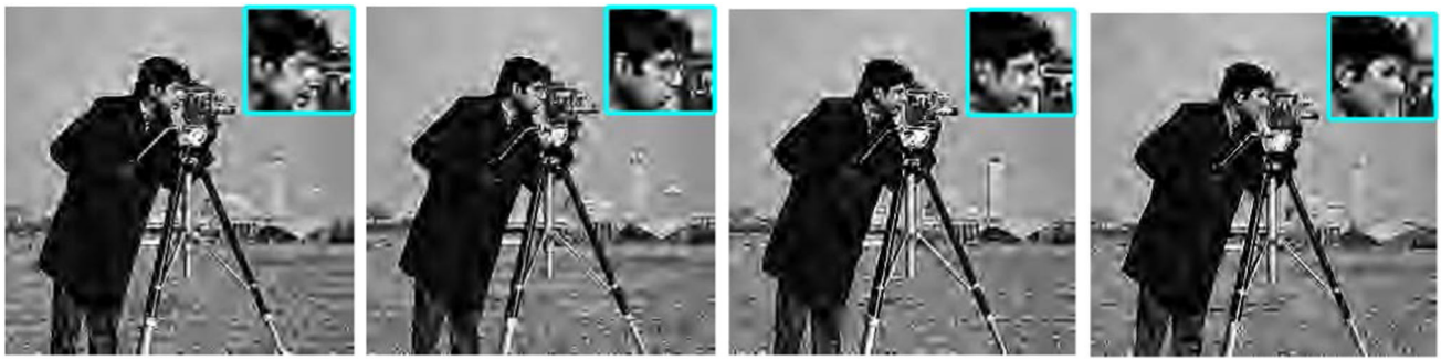
(a) 1-packet reconstruct. using packet #1 (23.04 dB) (b) 1-packet reconstruct. using packet #2 (23.02) (c) 1-packet reconstruct. using packet #3 (22.96 dB) (d) 1-packet reconstruct. using packet #4 (23.01 dB)
