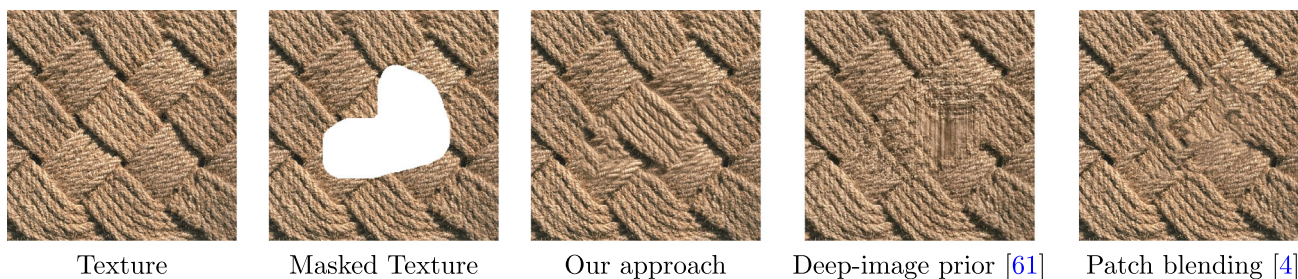
Fig. 17 Textural inpainting comparison. In this example, we compare our approach with Deep image prior [61] (which optimizes a deep neural network with skipping connection to generate the masked image using Mean Square Error criterion) and with [4], where patches from
