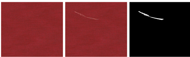
Fig. 4 A ground truth (on the right) for anomaly detection has been generated by introducing an anomaly in a RPN [50] texture (on the left), which is anomaly free. The detection is then done on the result (in the middle)
