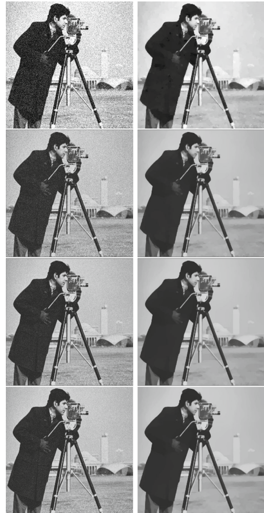
Fig. 5 Noisy (left) and denoised (right) images for classical \mathcal{DG}_0 on pixels (top row), and finite element solutions in \mathcal{DG}_0 (second row), \mathcal{DG}_1 (third row) and \mathcal{DG}_2 (bottom row) for (DTV-L2) with parameter \beta = 3 \times 10^{-4} in the isotropic setting ( s = 2 ). Results obtained using Algorithm 1 (split Bregman), see Table 4
