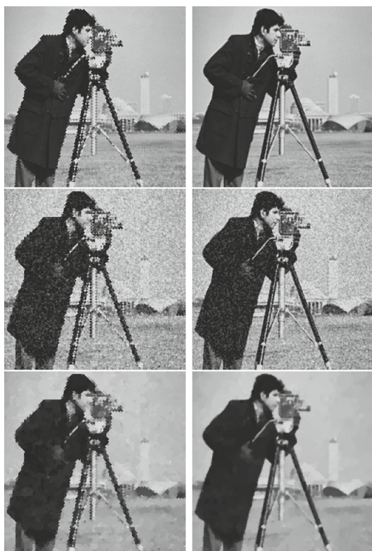
Fig. 6 Original (interpolated), noisy and denoised images (top to bottom) for \mathcal{DG}_0 (left column) and \mathcal{DG}_2 (right column) for (DTV-L2) with parameter \beta = 4 \times 10^{-4} for the isotropic setting ( s = 2 ) on a coarse grid. Results obtained using Algorithm 1 (split Bregman), see Table 5
